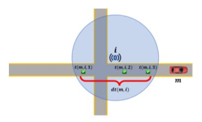
Figure 2. A vehicle detected many times at the same intersection.
