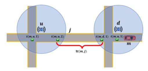
Figure 3. A vehicle detected by an upstream and downstream BS on a road.
