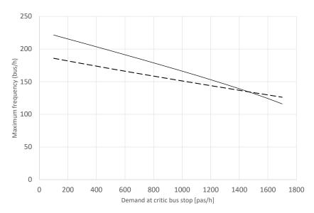
FIGURE 4 Capacity of bus corridor comparison between traditional (dashed line) and convoy (solid line) operation.
