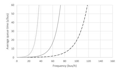
FIGURE 1 Average queue time data obtained from an IRENE simulation of a bus stop with one berth and three different dwell times: (i) 10 s/bus (dashed line), (ii) 20 s/bus (solid line), (iii) 40 s/bus (dotted line).
