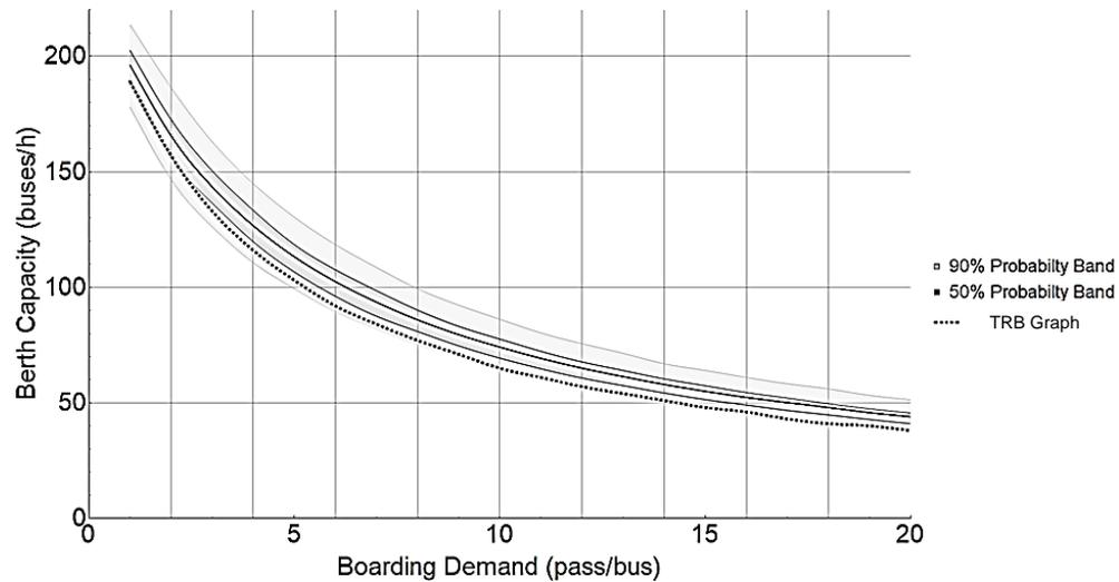
**Figure 6. Capacity of a bus stop as a function of the number of boarding passengers**
