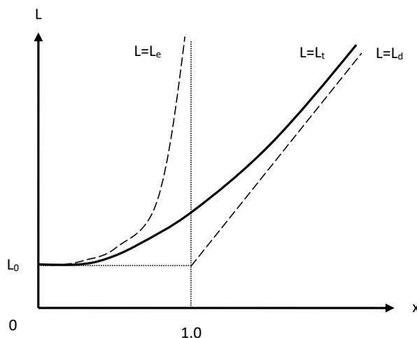
**Figure 2. Coordinate transformation function to calculate queue length at junctions.**
