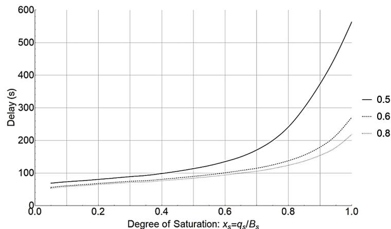
**Figure 9.** Delay as a function of  $(g/C)$  for  $C = 60$  s.
