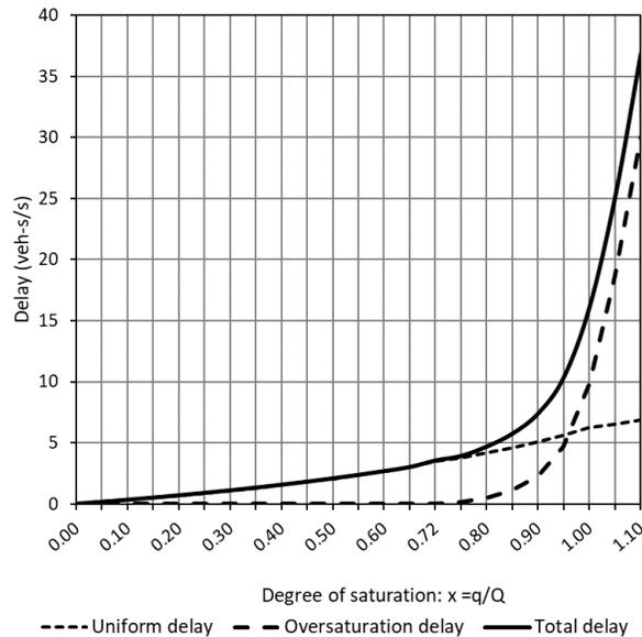
**Figure 1. Delay rate as a function of the degree of saturation at a signalised junction.**
