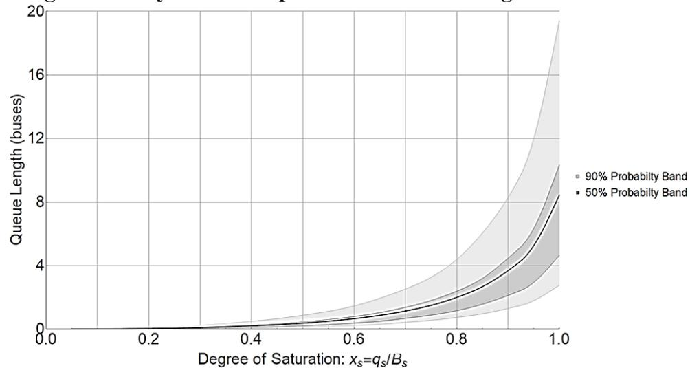
**Figure 8. Queue length in a bus stop as a function of the degree of saturation.**
