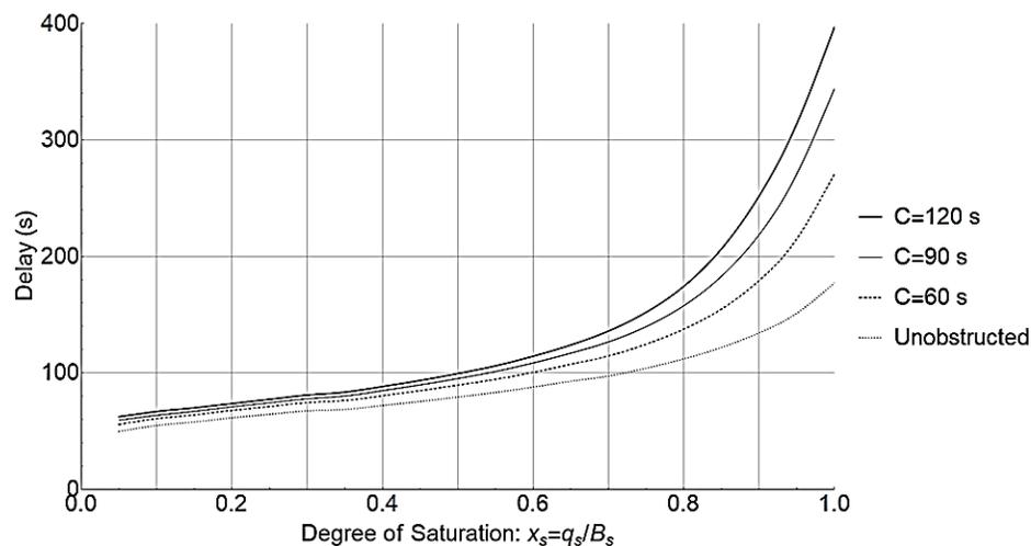
**Figure 8.** Delay as a function of the cycle time for  $(g/C) = 0.6$ .
