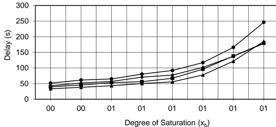
**Figure 4. Delay at a 2-berth bus stop.**
