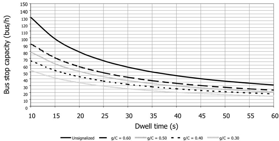
**Figure 3. Bus stop capacity with on-line berth (TRB, 2003)**
