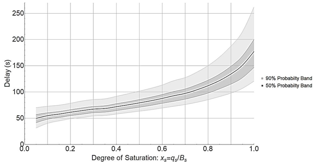
**Figure 7. Delay in a bus stop as a function of the degree of saturation.**
