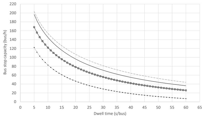
**FIGURE 2** Bus stop capacity considering two berths and an average queue time of 15 seconds per bus in three different cases: (i) isolated without an overtaking lane (solid line), (ii) isolated with an overtaking lane (dashed line), (iii) with a traffic light two bus lengths downstream and no overtaking lane (line with markers), (iv) with a traffic light immediately downstream and no overtaking lane (dotted line).
