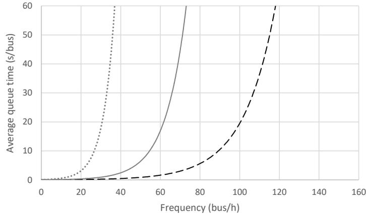
**FIGURE 1** Average queue time data obtained from an IRENE simulation of a bus stop with one berth and three different dwell times: (i) 10 s/bus (dashed line), (ii) 20 s/bus (solid line), (iii) 40 s/bus (dotted line).
