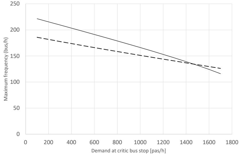
**FIGURE 4 Capacity of bus corridor comparison between traditional (dashed line) and convoy (solid line) operation.**
